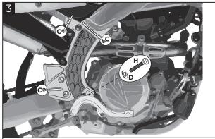
Place the X-Grip. Tighten the screw (H) and the washer (D). Fix them with the zip ties (C).
