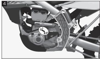
Place the X-Grip. Tighten the screw (I) and the washer (E). Fix
